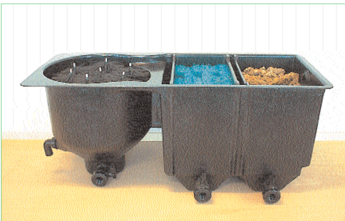
This 3-chamber-filter (amtra BIOPOND, Professional 15-3) is suited for ponds up to 15,000 ltrs. (with low fish population), and up to 12,000 ltrs. for a Koi populated pond. The first chamber as a Vortex contains brushes, the second chamber filter matting. The third chamber can be individually filled, with a maximum of 25 ltrs. (e.g. amtra CLINOP Zeolith 10 l GT 231). Thus the optimal water filtration is guaranteed. photo: amtra
